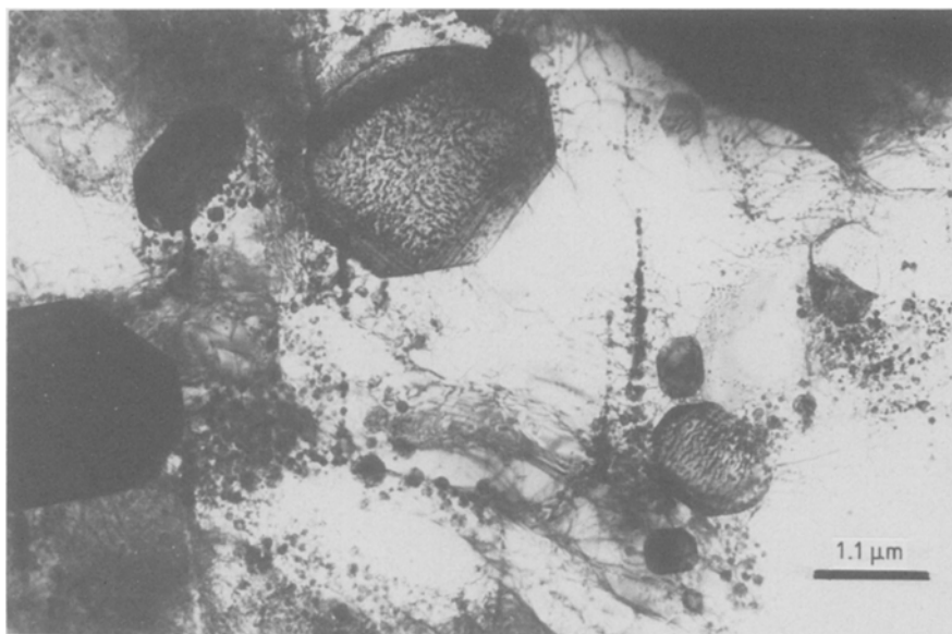
Figure 9 TEM bright-field image of a typical area in a reduced sample of Type 1. The dark lines are free dislocations in the MgO matrix. The bar is 1.1 μm.
